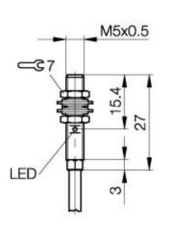
**Inductive Sensors** BES 516-3005-E4-C-PU-02 M5x0.5 x 27 normally-open Sn=0,8mm shielded
